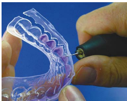
Figure 4. Using the twist drill HSS at high RPM (>20 000 rpm) trim around the gingival margins to achieve the final shape.
