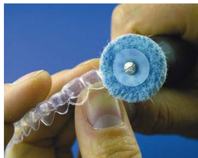
Figure 6. Finally smooth the edges of the tray with a silicon impregnated disc at low speed (<10 000 rpm). (Lisko-S part no. 22 32 10).
